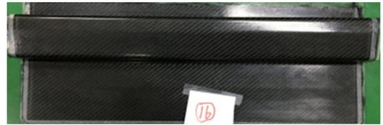
(b) Good in case of resin flow time, 1min
