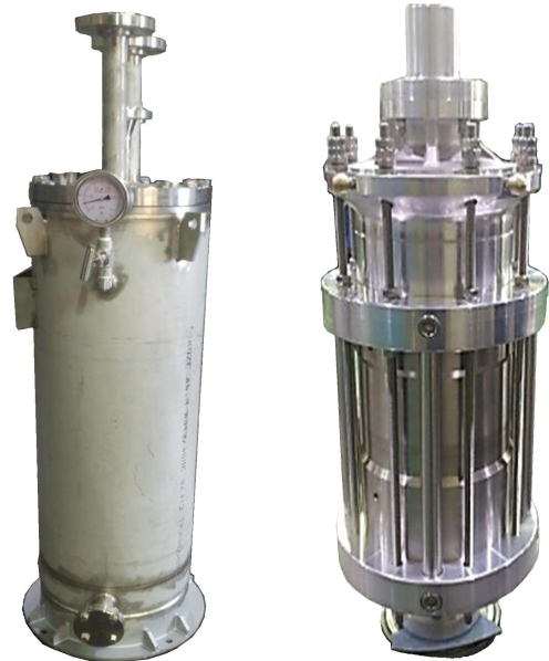
(a) Pump housing (b) submerged pump
