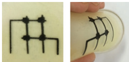
Fig. 3 Photograph of the direct-printed flexible tactile sensor element
