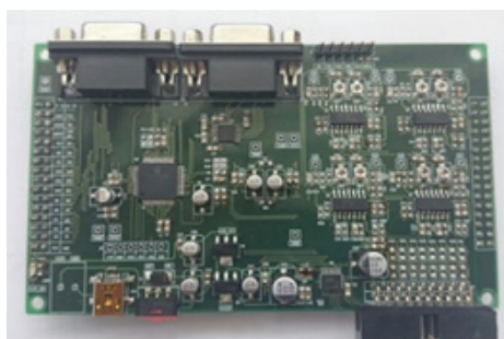
Fig. 6 Photograph of analog-signal-processing module for direct-printed flexible tactile sensor
