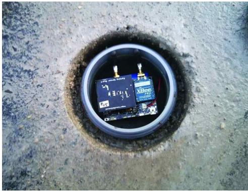
[Fig. 1] A sensor placed in the parking area
