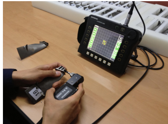
Fig. 4 Experiment set up for eddy current inspection data acquisition
