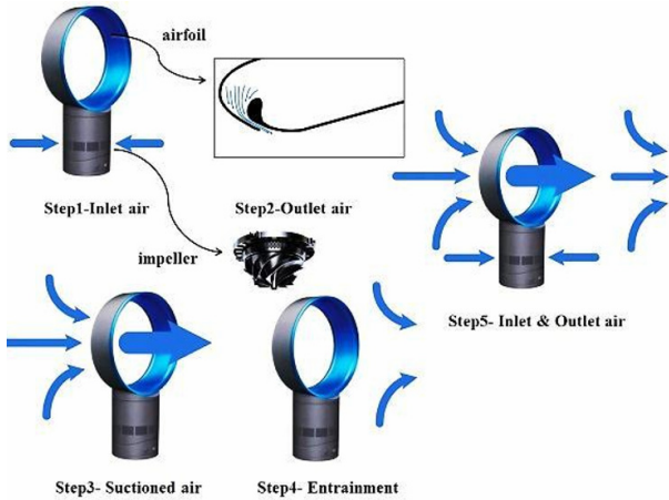
Fig. 2 Mechanism of bladeless fan (9)
