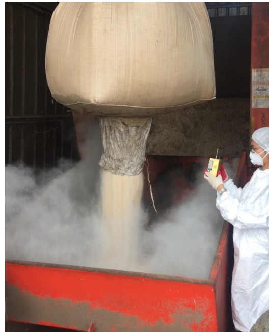
(b) Measuring of inhalable and respirable dust concentration
