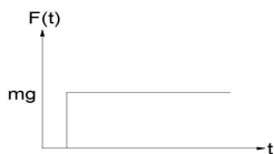
[Fig. 3] Impact load applied to strain-gage test
