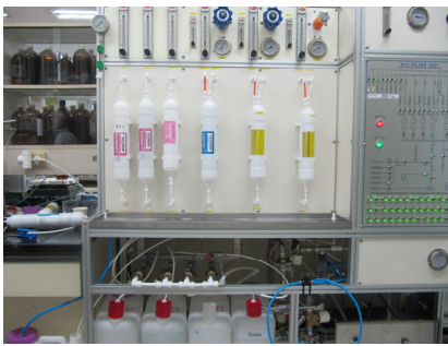
Fig. 2. Cleaning apparatus of used RO membrane filter.
