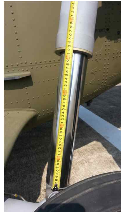
Fig. 4. Measure of length for chrome plating
