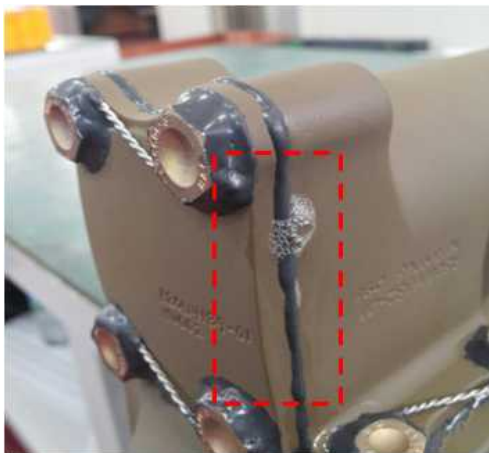
Fig. 6. External gas leakage
