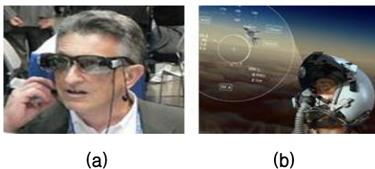
Fig. 1. (a) Civilian goggle display, (b) Pilot's Helmet Mounted Display
