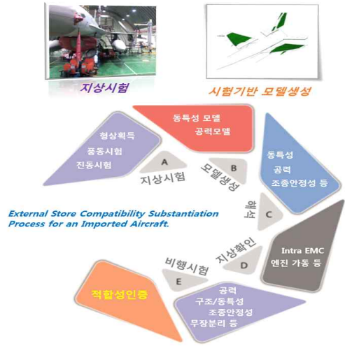
Fig. 1. External Store Compatibility Substantiation Process for an Imported Aircraft
