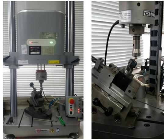
**Fig. 3** Fatigue testing machine for tests (electropuls E3000, instron inc., UK)
