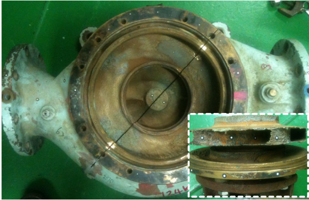
Fig. 4. Cut model pump for reverse engineering.
