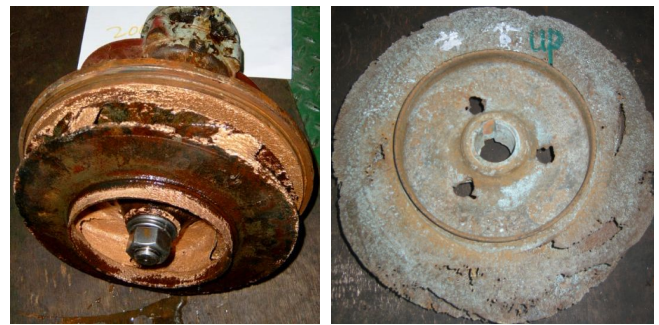
Fig. 3. Damaged impeller from model pump.
