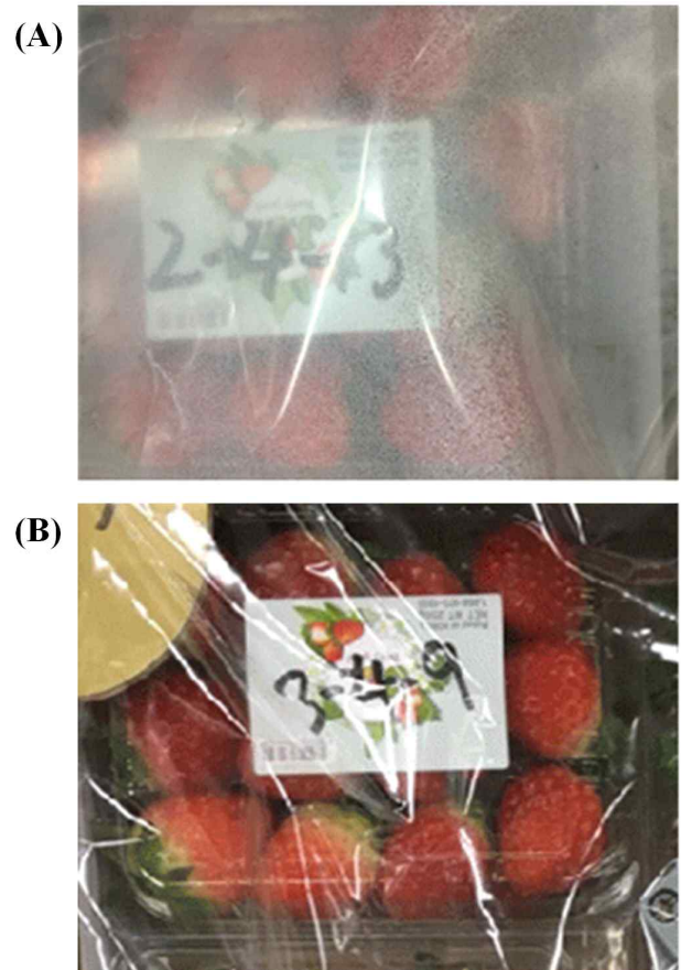
Fig. 3. Water condensation of MAP using LDPE and no condensation of MAP using PA film (B).
