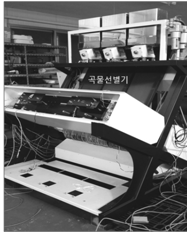
Fig. 6. Grain sorter NIR image board system
