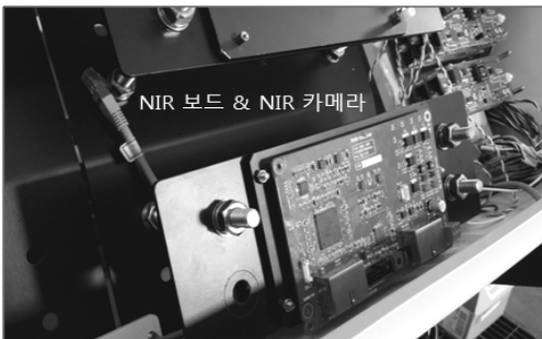
Fig. 5. NIR board and camera system
