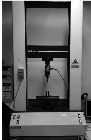
Figure 4. Test of flexural strength on UTM.
