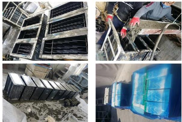
Fig. 8. Manufacture of composite specimens
