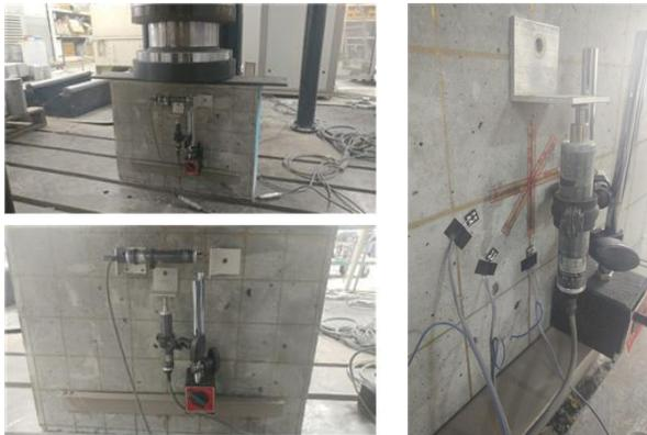
Fig. 9. Compression test with measurements
