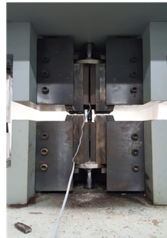
Fig. 8. Photo of tensile strength test
