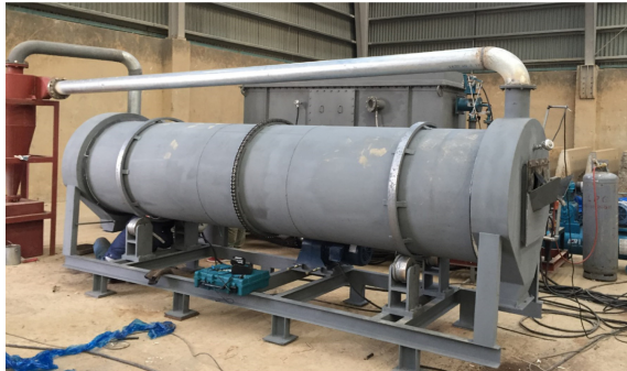
Fig. 3. Rotary kiln for drying contaminated ballast and desorbing some contaminants from the surface of ballast.
