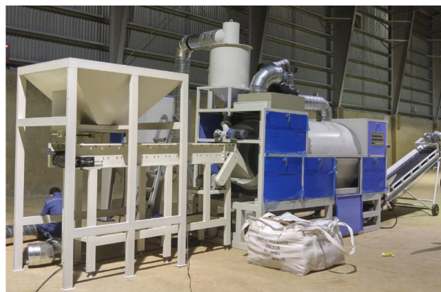
Fig. 5. Continuous-type dry washing equipment for gravel.
