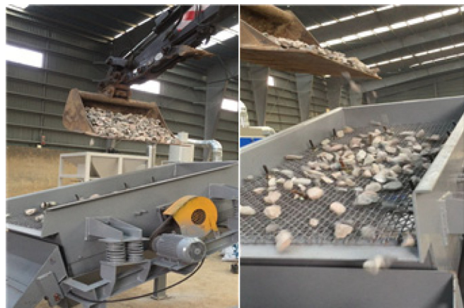
Fig. 6. Testing the performance of screen equipment.
