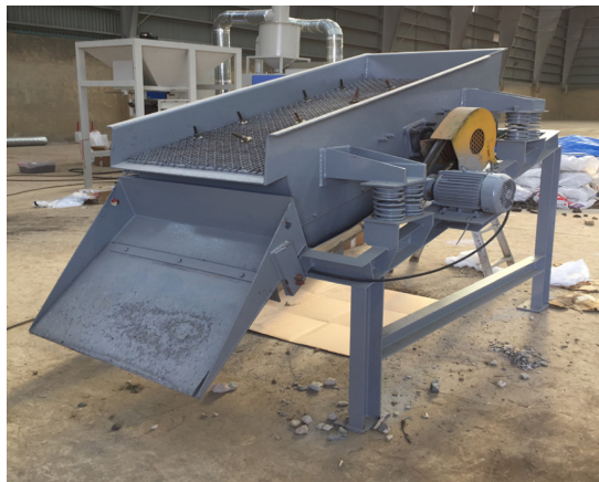
Fig. 2. Separator used in this study to collect ballast gravel pieces larger than 20mm.
