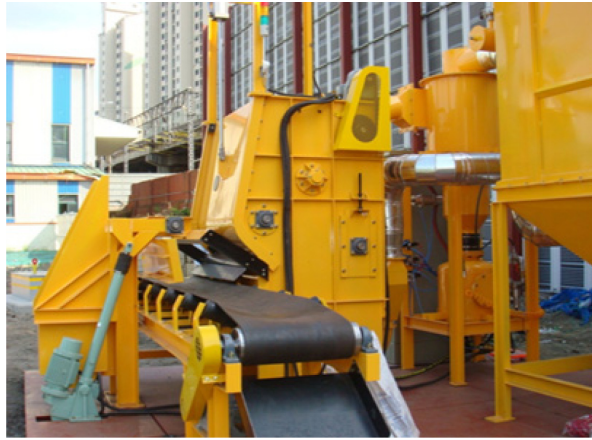
Fig. 1. Batch-type dry washing equipment for gravel.
