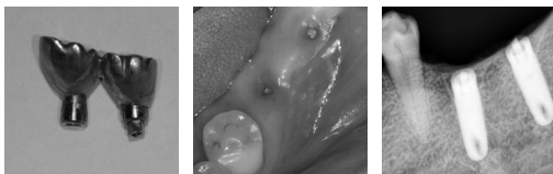
Fig. 1 The example for dental implant abutment fracture by screw loosening
