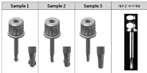
Fig. 8 Implant screw driver design (experimental/sample1-3, control group/ 'O' company)
