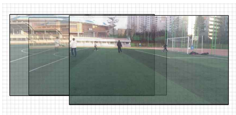
(e) Warped current Frames of V_1, V_2, V_3 aligned to the position of the previous Frame Fig. 7 Transformation of the Video Frames according to the proposed algorithm.
