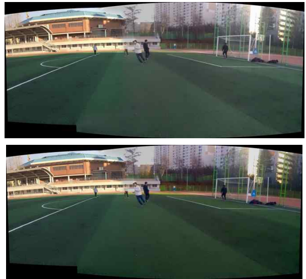
Fig. 6 Color Transfer based Color matching (top: Left Video Frame (iPhone 6 plus), Right Video Frame (HTC One M8), middle: Stitched Video Frame without Color Transfer. bottom: Stitched Video Frame applying Color Transfer)
