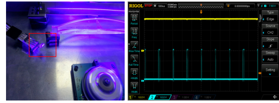
Fig. 6 One cycle time measurement of polygon mirror
