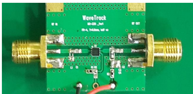
Fig. 4. Photograph of the plastic DFN packaged LNA MMIC and evaluation board.
