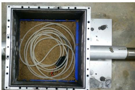
(a) Heating wire and 5TE sensor
