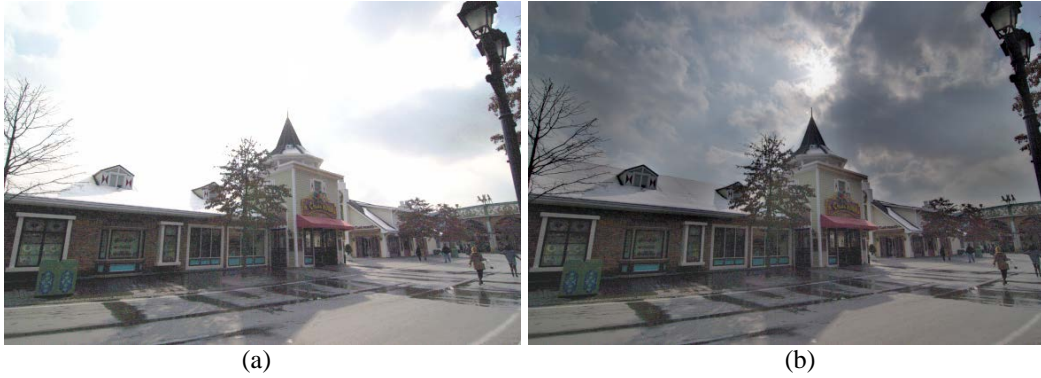
Fig. 3. Color calibration result using our method. (a) Histogram matching result I_h^S using Fig. 1 (a) and Fig. 1 (b) as the input image pair. (b) Exposure fusion result J^S using Fig. 3 (a) and Fig. 1 (b).
