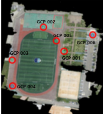
Fig. 10. Point cloud and GCP using Image
