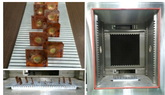
Fig. 5 Vertically aligned samples for copper corrosion test in temperature & humidity chamber
