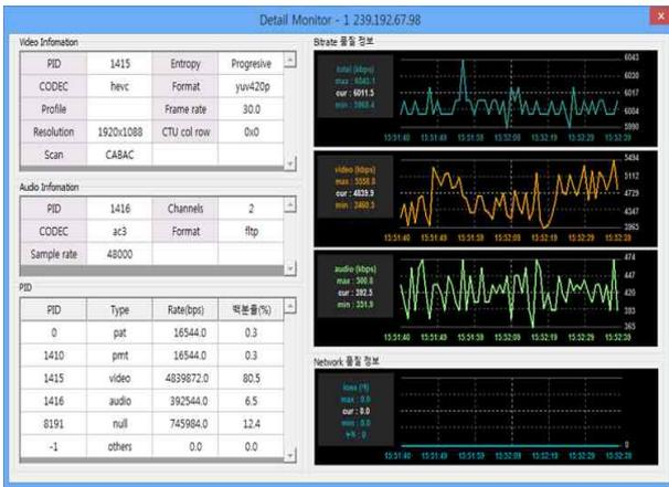
Fig. 11. Monitor video, audio, and quality of broadcast channels[5]
