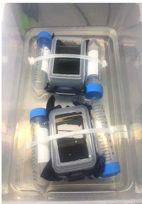
Figure 1. Photograph of 100 mL floating photobioreactors with PET meshes.
