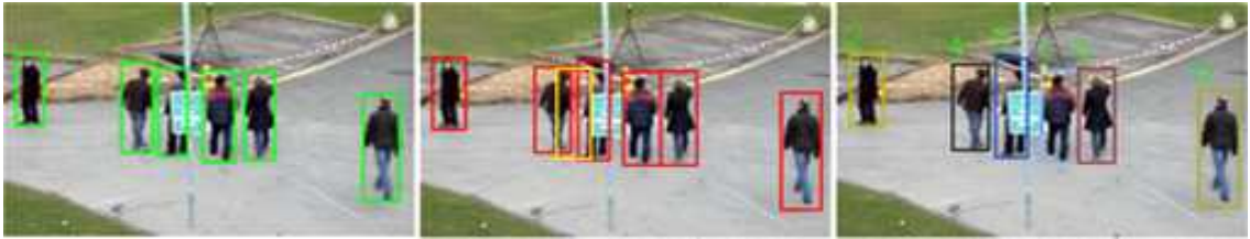
Fig. 3. YLSSOD's result, ground truth and tracking result at frame 86 of PET'09 S2.L1. (a) Ground truth (b) YLSSOD detection result (c) Tracking result of the proposed method
