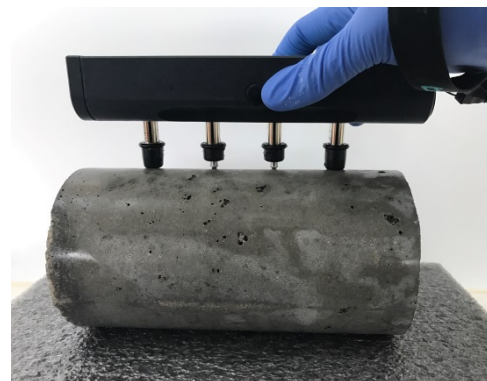
Fig. 4 Picture of surface electrical resistivity test
