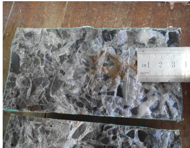
FIGURE II Measurement of Depth of Chloride Penetration
