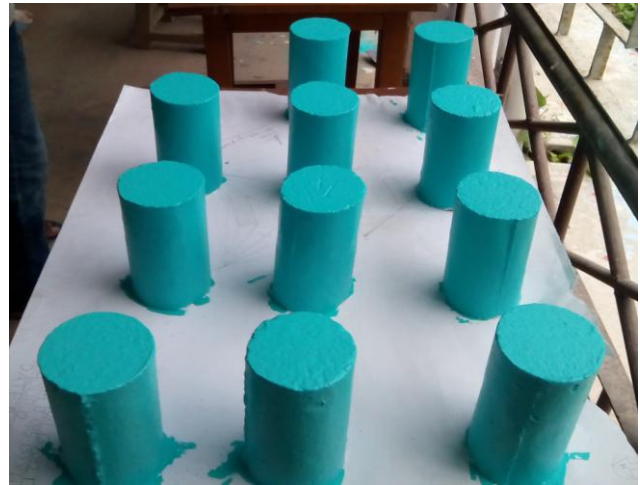
FIGURE I Preparation of Specimen for Salt Ponding
