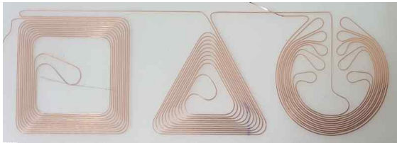
(b) Microforming pattern by ultrasonic vibration
