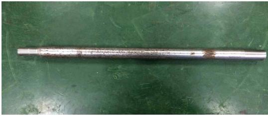
Fig. 11 Specimen with bruise defects
