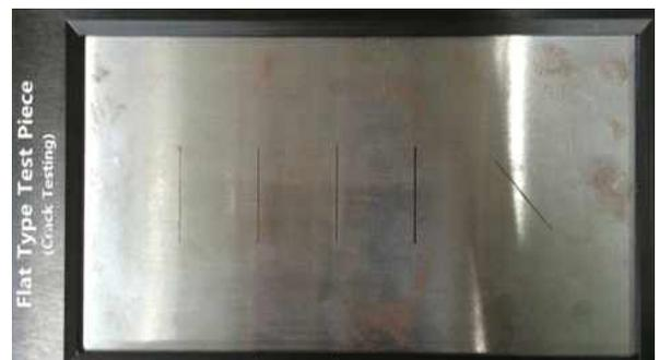
Fig. 10 Specimens with artificial cracks
