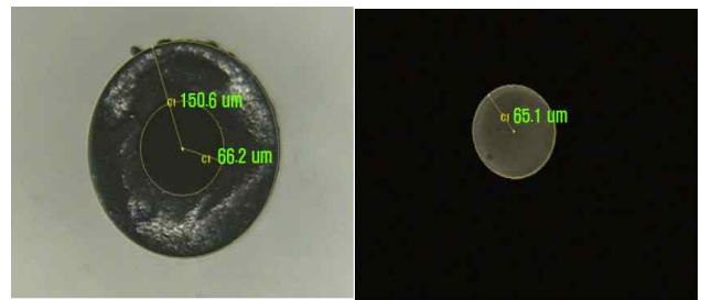
Fig. 14 The picture of the hole after 3 rd machining process
