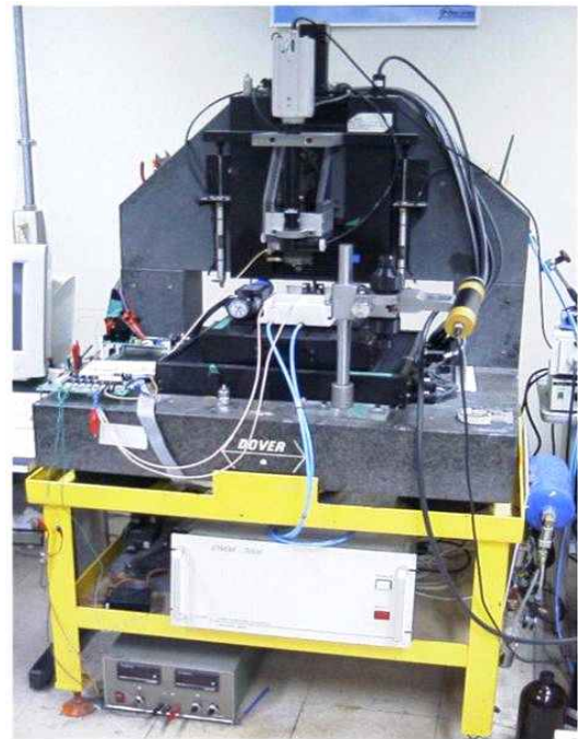
Fig. 1 Experimental set-up to manufacture micro-needle using micro EDM
