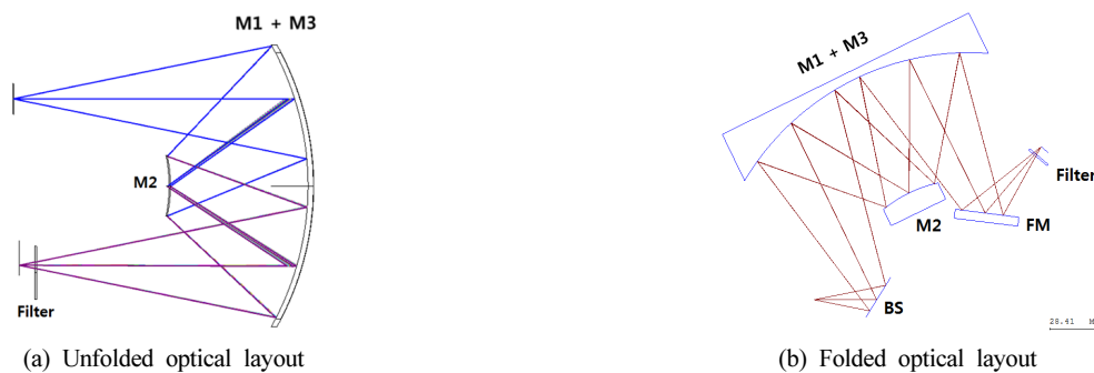
Fig. 4. Unfolded and folded optical layouts of the VNIR spectrometer.
