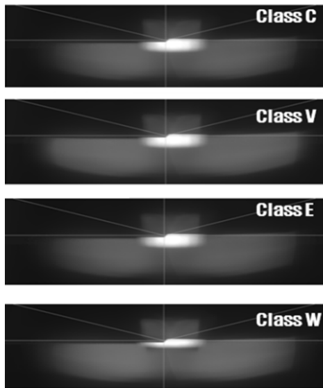
FIG. 12. Four beam patterns (Class C/V/E/W) formed by the left and right AFS systems together at a screen situated 25 m away.
