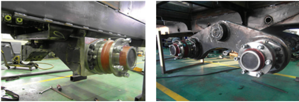
Figure 3. Front and rear wheel part of chip-harvester.
