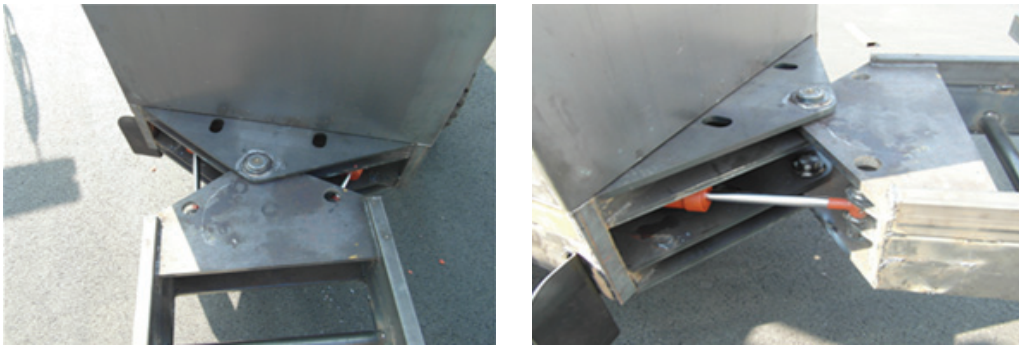
Figure 4. Articulate body of chip-harvester.
