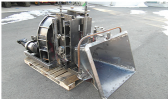
Figure 5. Chipper part of chip-harvester.
