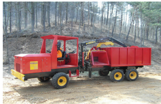
Figure 6. Shape of the developed chip-harvester.
