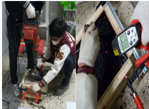
Production of HMA-Surface
