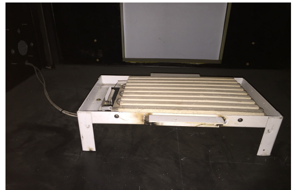
Fig. 4 Electrical heater installed the floor of a measuring chamber.
