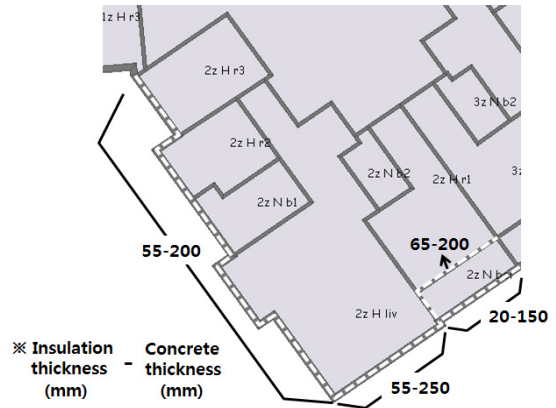
Fig. 9 No.202 external wall composition.
