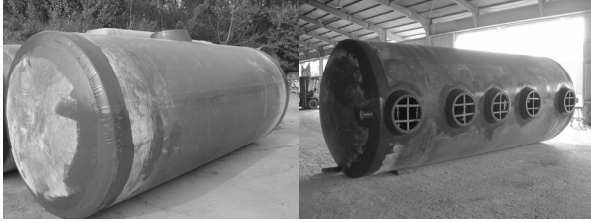
Fig. 2. GFRP septic tank
