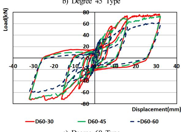
Fig. 3. Load-displacement relationship
