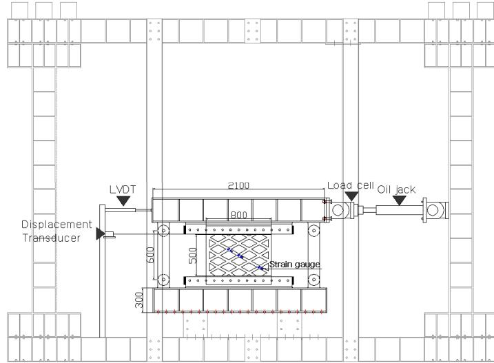
**Fig. 1.** Set-up of specimen
