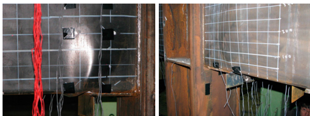
Fig. 6. Examples of web local buckling observed in the existing tests
