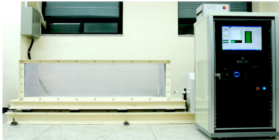
(a) System of Shaking Table Test
