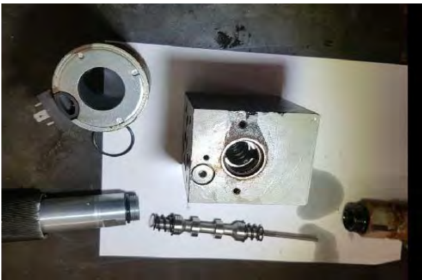
Figure 9: Disassembly investigation of clutch control solenoid valve
