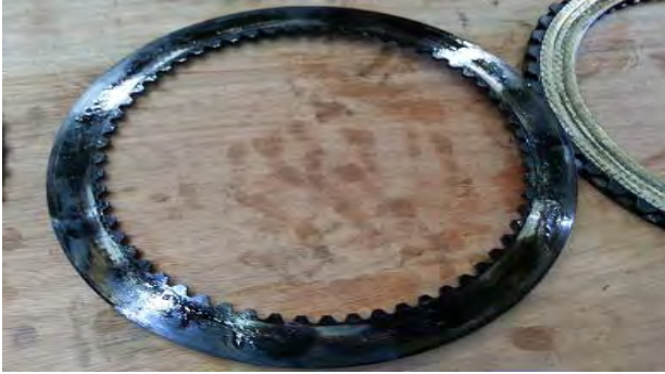
Figure 7: Damaged pair of inner and outer plates
