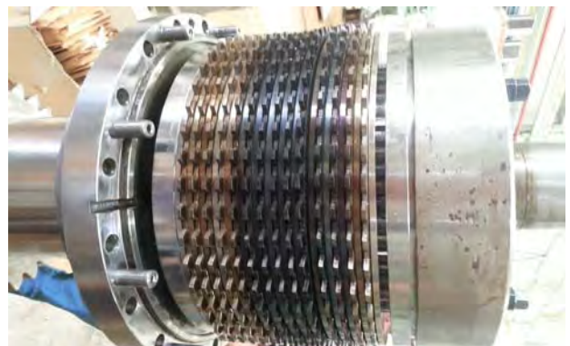
Figure 6: Sticking of the clutch assembly
