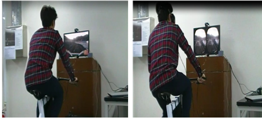
Fig. 2. VR bicycle device designed for experiment (Left : 2D, Right : HMD-based VR)
