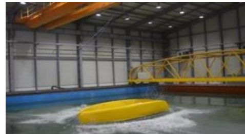
Fig. 5. Photographs of Leisure boat's drop test in RIMS's square tank
