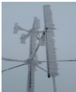
Fig. 2. Hard rime of antenna
